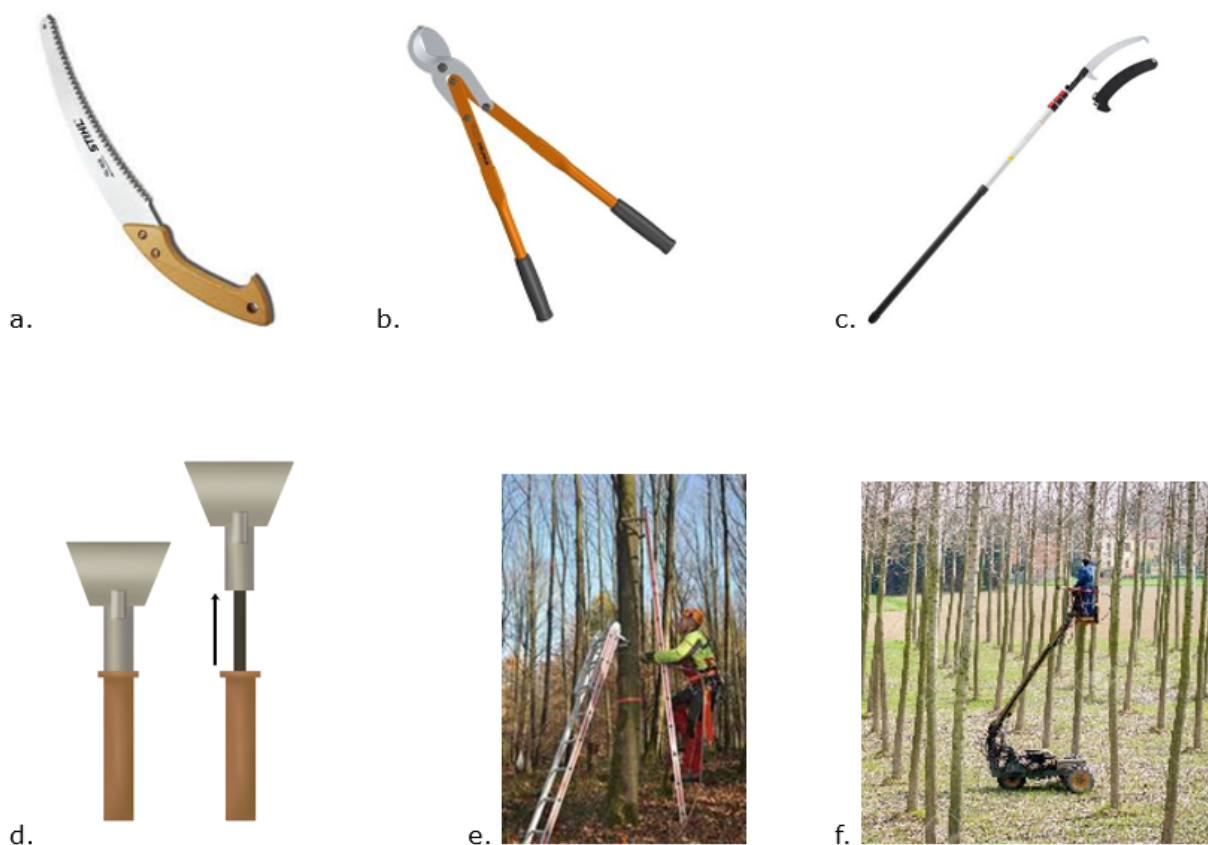
Fig. 44-7: Common tools used for pruning as a silvicultural intervention (a. pruning saw, b. pruner, c. pole saw, d. pruning chisel, e. pruning ladder, f. cherry picker platform)
