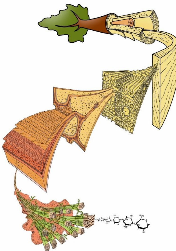
Figure 12-7: The structure of wood in a tree at different levels, ranging from the basic constituent cellulose, that is arranged in microfibrils which form a composite with hemicellulose and lignin in the multi-layered cell wall which constitutes the dead cells, but also forms an essential part of living cells. The many dead and few living cells (radial and sometimes axial parenchyma) constitute the xylem. The xylem is organised in growth rings reflecting its way of formation through time. In case of tree species growing under a seasonal climate with one pronounced growing season and one dormant season, annual tree rings are formed. With aging of the tree and increasing tree-ring number xylem structure slightly changes; moreover, secondary changes of the xylem such as heartwood formation can occur in some species making that the wood structure along and across the stem is not homogeneous. Adapted from M. Harrington, University of Canterbury.
