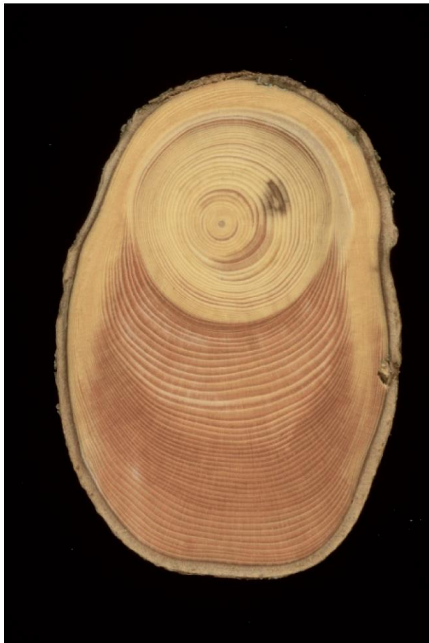
Figure 12-18b: Reaction wood in spruce. The tree once experienced tilting due to wind, and has since produced compression wood (left). The microscopic image of the compression wood (right) exhibits highly thickened cell walls of tracheids with large intracellular spaces among the cells (magnified 400 times). Photos taken by Fritz Schweingruber.
