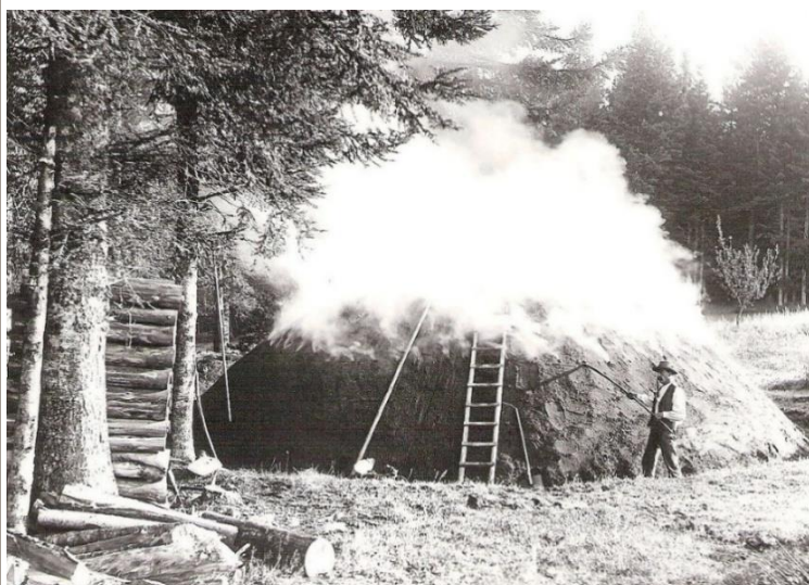
Photo Box 46.1.1. A charcoal kiln in full operation in the German Black Forest around 1910. By making holes in the layer of earth over the kiln, the oxygen supply and the temperature in the burning kiln can be accurately controlled. Photo: Karl Blumenthal.
